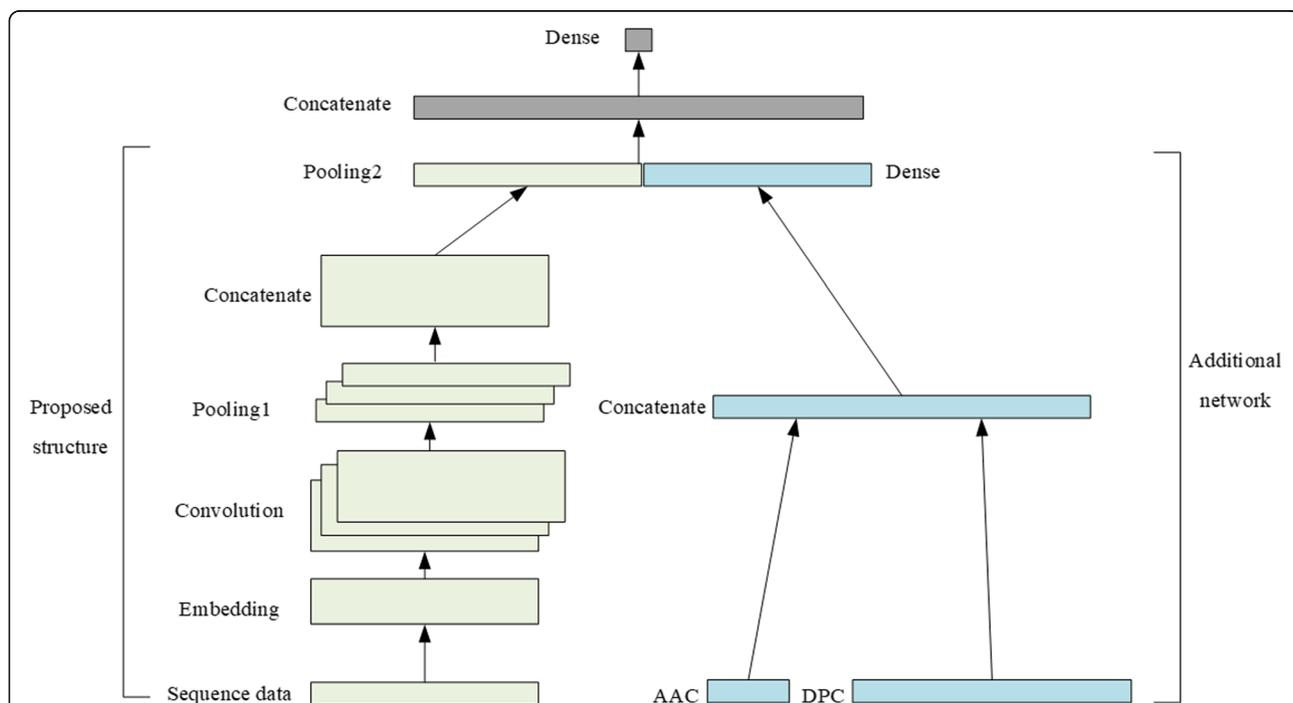
**Fig. 4** The structure of the proposed fusion model. There are two parts in the fusion model. The proposed structure is on the left. An additional fully connected network is on the right and this part make use of the DPC and AAC of peptide sequences. This network incorporates redundant information into the proposed model
