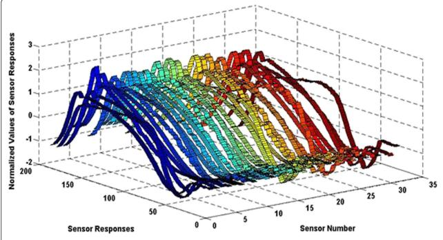
**Figure 2** Signal response for odour recognition. A surface plot shows the visualized data for single bacteria samples gathered using a Cyranose320 e-nose system.
