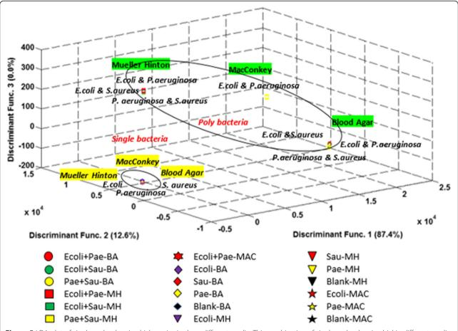
**Figure 5** LDA plot of single and poly microbial species in three different media. This combination of single and poly microbial in different media is to study the effectiveness of e-nose to classify the bacteria in a different group region.
