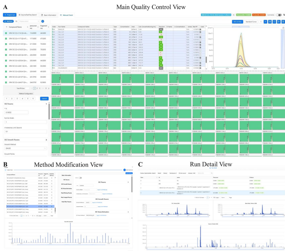
Fig. 2 The main views of manual inspection is also the main operating panel of MRMPPro. A The main operation panel of MRMPPro includes a series of functions such as peak selection calibration, integration calibration, concentration curve calibration, identification state inspection, etc. B Method parameter configuration view. C The detailed view of every raw file. It allows researchers to view the metadata information and each chromatogram data
