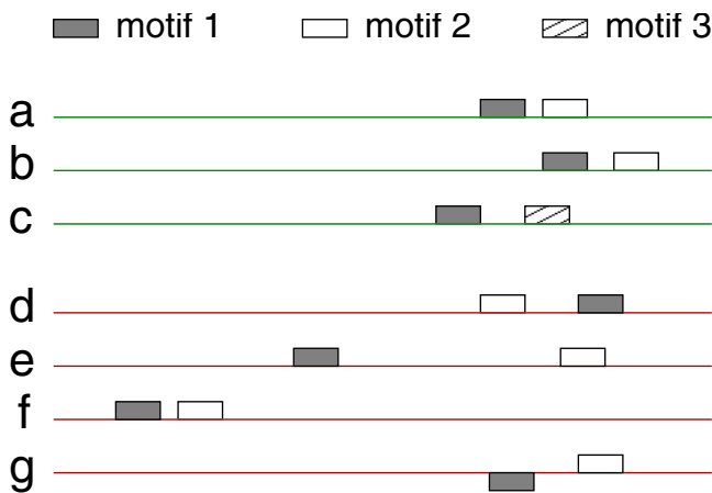
Figure 1 Example CRM Learning Task. An example of a CRM learning task: There are three types of transcription factor binding sites on these DNA sequences. Transcription will occur in a given condition if motif 1 is followed closely by either motif 2 or motif 3 near the transcription start site (right side) on the sense DNA strand. This is true for sequences a , b , c , but not sequences d (incorrect order), e (too far apart), f (too far upstream), and g (motif 1 on the incorrect DNA strand).
